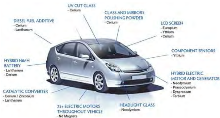
Figure 2.2 Examples of Rare Earth Metals used in an electric vehicle 21
