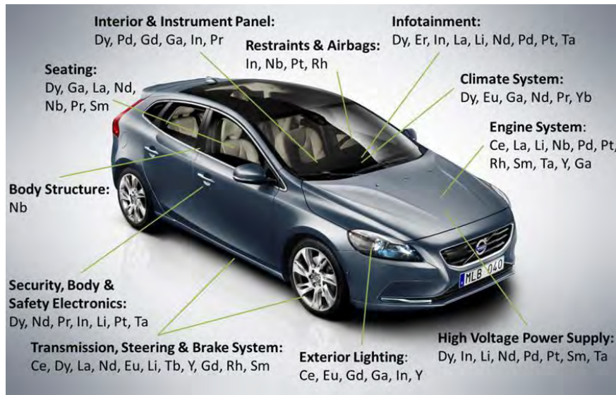
Figure 4.1 Summary of the results from the detailed analysis in terms of distribution by subsystem. Showing where the 24 materials' main masses were identified. The figure is a summary of all 4 analysed cars 143
