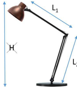
Luminaire (articulated) External dimension: the larger value of L_1 or L_2 , (not value H)
